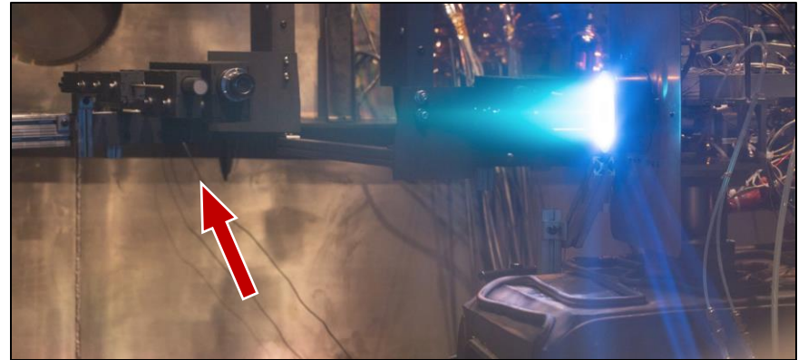
Far-Field Probes (left) and HET-X thruster (right)
