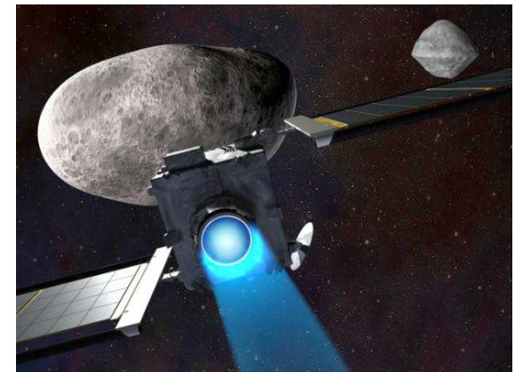
Electric thruster used for NASA's DART mission
